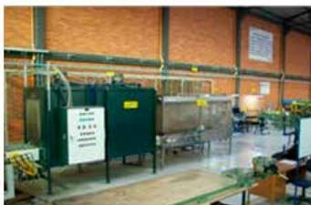
*Thermoforming process for plastic pipes*
