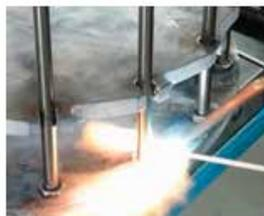
*Brass Brazing Process for hydraulics lines*
